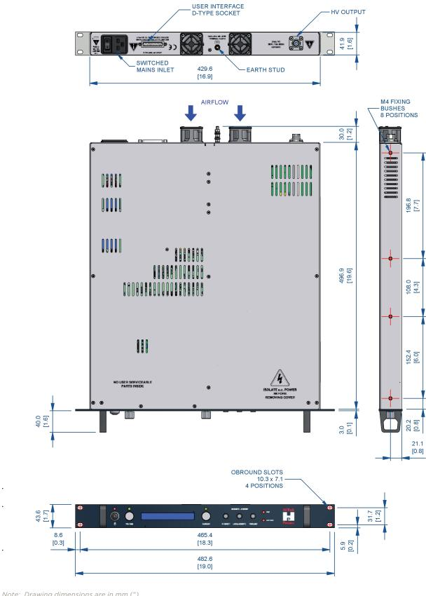
Note: Drawing dimensions are in mm (")
